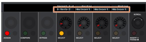
8. Press the ninth [Multi function button A] from the left or the one that corresponds to the channel with insert. The selected insert is assigned.
