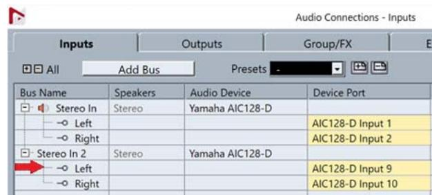
If an input bus with multiple channels (such as stereo or surround channels) has been assigned, the parameters for the bus channel appearing first in Nuendo's “Audio Connections” (“Left” for a stereo channel) are shown in the label area.
