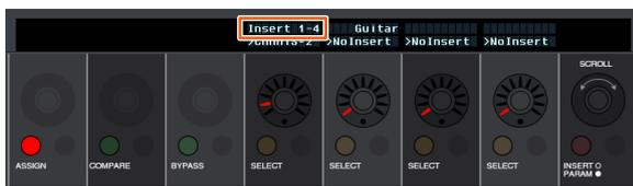
7. Turn the [Multi function knob] to select the insert. The [Multi function knob] to be operated varies depending on the target slot for “Insert.”
