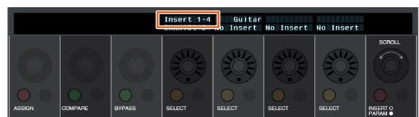
5. Press the [Multi function button A] that corresponds to the “Insert” you want to change the parameters of.
