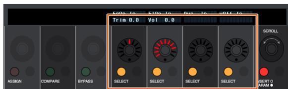
7. Turn the [Multi function knob] or press the [Multi function button] corresponding to the parameter and change the parameter’s value. The value you change to will immediately be applied.
