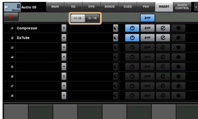
The tab switches between insert slots 1 – 8 and 9 – 16.
