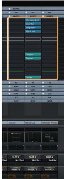
The insert slots on the channel strips can be selected using [▲][▼] in the SECTION CONTROL section.
