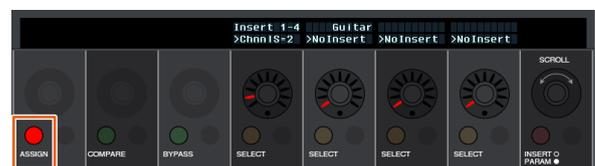
6. Turn the 16th [Multi function knob] from the left of the Nuage Fader CHANNEL STRIP section (the far right knob), then select from group A – D or E for which insert is used. “Insert 1 – 4” (A – D) or “Insert 5” (E) will be displayed on the Plug-in Panel window.
