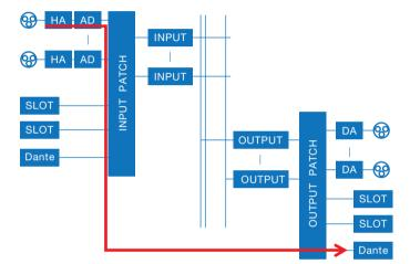
Use the PORT TO PORT function to output from an input jack on the rear panel to a Dante connector without sending the signal through the mixer. This allows you to use the I/O jacks on QL series consoles as I/O jacks for an audio network.
