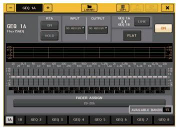
This window is the same as that for the 31BandGEQ, except that the AVAILABLE BANDS parameter box indicates the real-time number of additional bands (maximum 15) that can be controlled in the current GEQ.
