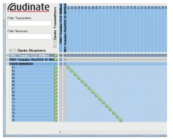
In this case, you'll need to switch the DANTE INPUT PATCH settings of the QL series console depending on whether you're performing multitrack recording or multitrack playback. If you've saved these different sets of settings in the DANTE INPUT PATCH LIBRARY (page 150), you'll be able to switch between them conveniently.
