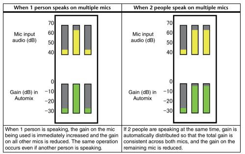
The Dugan speech system functions differently from a limiter or auto level controller. When multiple people are speaking, the engineer can adjust each level using the faders as normal. Even if nobody is speaking, the system searches for mic audio and automatically distributes gain. Therefore, faders can leave in their raised positions.
