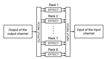
Alternatively, you can assign the input and output of the internal effect to the insert-out/in of a desired channel (except for a ST IN channel), so that the effect is inserted into that channel.
