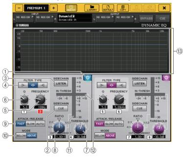
(1) **BAND ON/OFF button** Turns each band on or off.
