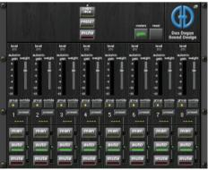
Press this area to open the AUTOMIXER EDIT window, in which you can modify the automixer settings.
