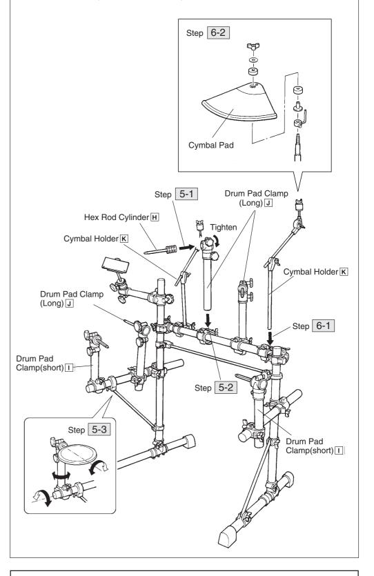
After the above assembly is complete, set the Kick Pad, Hi-Hat Control Pedal, etc. into position and connect the necessary cables. To keep cable out of the way while playing, use the supplied Cable Bands to hold the cables to the rack systems's pipes.
