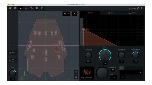
Use the Master Gain knob at the bottom to adjust the overall output level of the 3D Reverb. And with the Zone option next to the Master Gain knob, select a zone to determine which zone the 3D Reverb is output.
