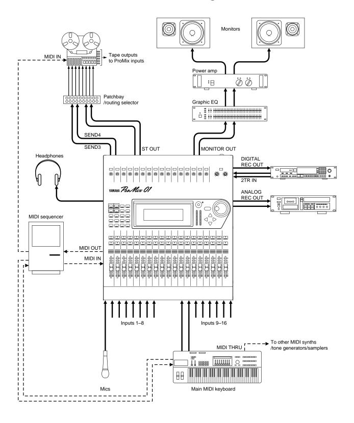
This example shows ProMix 01 in a multitrack recording application. It is basically the same as the MIDI Studio application with the addition of a multitrack recorder. Although not specifically designed for use as a recording mixer, multitrack recording with ProMix 01 is possible with a little patching. In the illustration, an analog multitrack tape recorder is shown. This could, however, just as well be a hard disk recorder.
