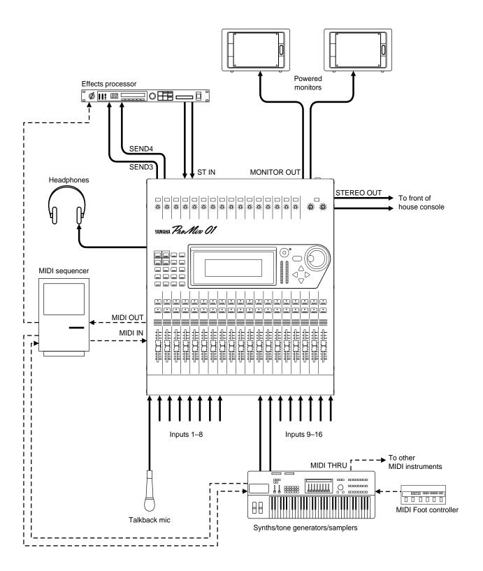
This example shows ProMix 01 in an onstage keyboard mixing application. Line-level sources are connected directly to inputs channel 9 through 16. With the correct connectors, line-level sources can also be connected to input channels 1 through 8. Balanced microphones for foldback or miking up a rotary-type speaker cabinet can also be connected.
