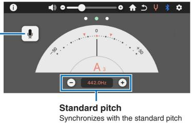
Synchronizes with the standard pitch setting of the HD-300.
