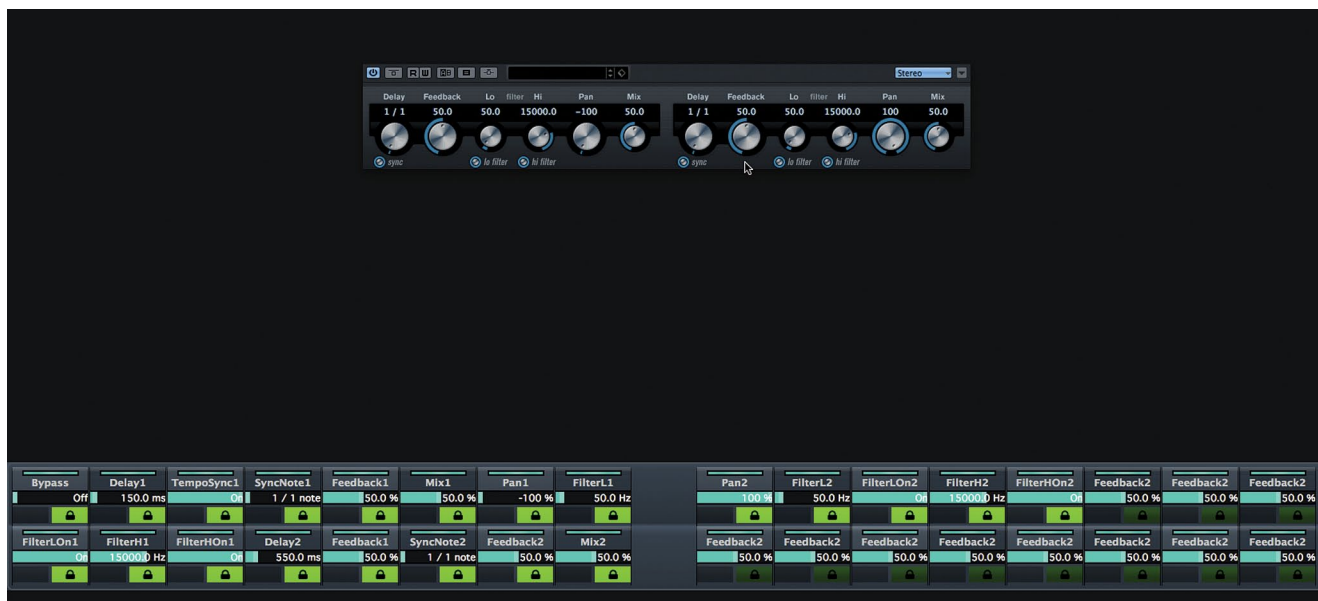
Figure 7.12 Freely assigning parameters to unlocked knobs
