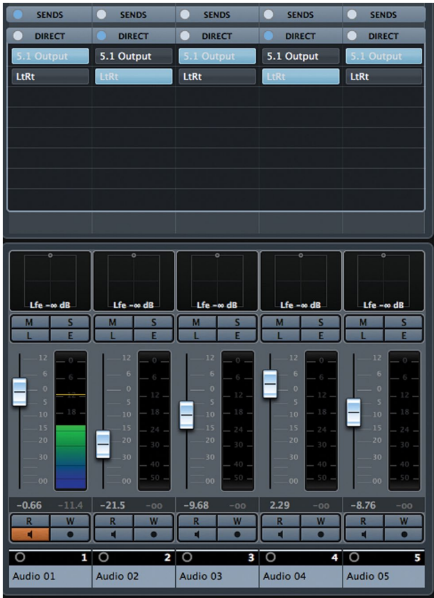
Figure 6.81 Direct Routing rack
