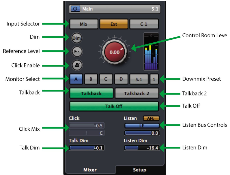
Figure 4.38 Control Room Main section
