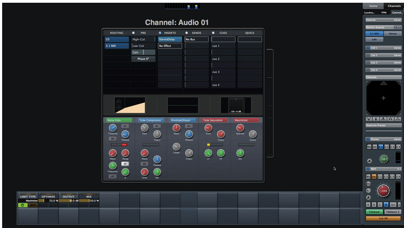
Figure 7.7 Slot 2 showing the limiter
