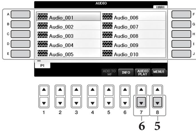
5 Call up MENU1 at the right bottom of the display by pressing the [8▼] button as necessary.
