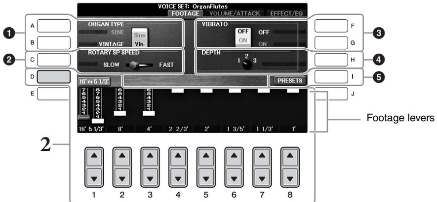
If you want, you can select the Organ type, change the Rotary Speaker speed and adjust the Vibrato setting, by using the [A] - [C] and [F] - [H] buttons.
