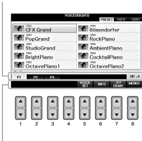
If a menu appears in this section of the display, use the [1▼] – [8▼] (lower) buttons to select the desired items.
