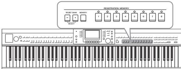
The Registration Memory function allows you to save (or “register”) virtually all panel settings to a Registration Memory button, and then instantly recall your custom panel settings by simply pressing a single button. The registered settings for eight Registration Memory buttons should be saved as a single Bank (file).
