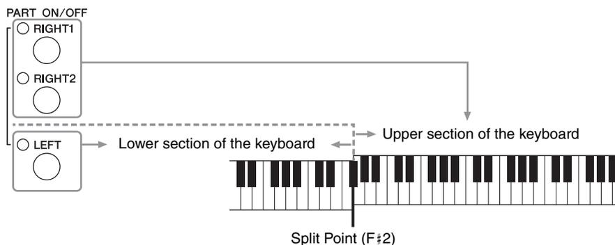
When the LEFT part is off, the RIGHT1 and 2 Voices can be played over the entire keyboard. When the LEFT part is on, keys lower than F#2 (the Split Point) are set for playing the LEFT part and those higher than the Split Point are set for playing the RIGHT1 and 2 parts. The lamp of the Split Point (at which the keyboard is divided into the right and left sections) lights. The Split Point can be changed (page 69).
