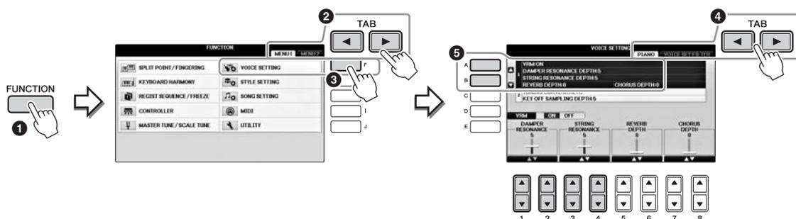
Use [D] button for turning the VRM function on or off, or use the [1▲▼][2▲▼] buttons for adjusting the depth of damper resonance and the [3▲▼][4▲▼] buttons for that of string resonance.
