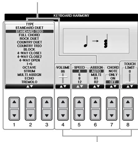
If a parameter appears in slider (or knob) form, use the [1▲▼] – [8▲▼] buttons to adjust the value.
