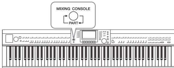
The Mixing Console gives you intuitive control over various sonic aspects of the keyboard parts and Song/Style channels, including volume balance and the timbre of the sounds. It lets you adjust the levels and stereo position (pan) of each Voice to set the optimum balance and stereo image, and lets you set how the effects are applied.
