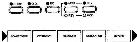
If, however, you only wanted to use the compressor, equalizer and reverb stages, you could press the O.D. and MOD keys to turn the stages OFF, resulting in the effect chain shown below:
