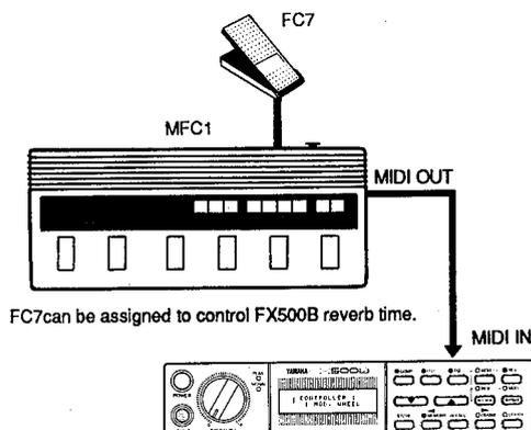
In order to use this kind of setup, the two "controllers" that the FX500B allows — CONTROLLER 1 and CONTROLLER 2 — must be set to receive specific MIDI CONTROL CHANGE data (i.e. receive data from a specific MIDI controller) using the Control Change 1 Table Edit and Control Change 2 Table Edit functions described below.
