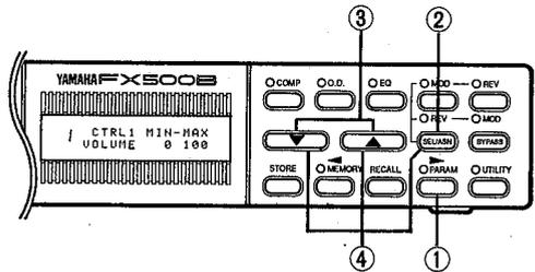
Once the MIDI controllers you wish to use have been selected using the Control Change 1 Table Edit and Control Change 2 Table Edit functions described above, you can then assign the controllers to the specific FX500B effect parameters. Control assignment is carried out in the PARAM mode.
