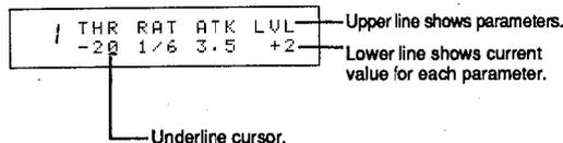
The PARAM mode can not be directly selected from the UTILITY mode by pressing the PARAM key. The UTILITY mode must first be exited by pressing several times or holding (about one second) the UTILITY key until the UTILITY key indicator goes out.
