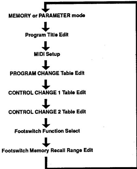
The mode that was active before the UTILITY key was pressed (MEMORY or PARAM) is selected following the last function on the utility list. The UTILITY mode can also be exited by pressing and holding the UTILITY key until the UTILITY key indicator goes out (approximately 1 second).
