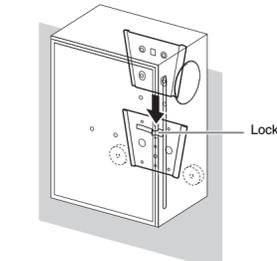
To detach the mounting bracket from the bracket base, release the lock of the mounting bracket with a long flat-blade driver and lift the speaker.
