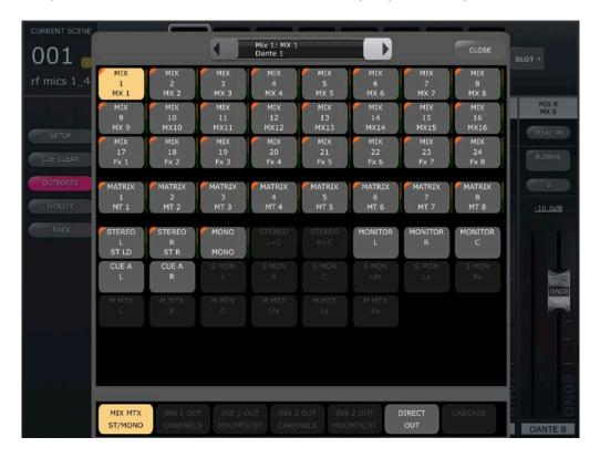
If there is a current assigned patch, this will be displayed in the patch view on the patch button grid, and shown in the top line of the small window at the centre-top of the patch view the second line will display the currently selected output port.
