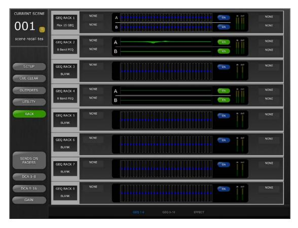
Tabs at the bottom of the screen provide access to the GEQ 1-8, GEQ 9-16, and the EFFECT racks.
