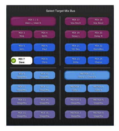
Select the Target from Mix 1-24 and Matrix 1-8. The currently selected Mix will appear as a white button with a check mark. Stereo pairs appear as single large buttons.
