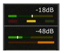
Dynamics 1 is displayed at the top of the thumbnail with Dynamics 2 at the bottom. (Output channels have only Dynamics 1.)
