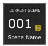
The Scene Memory area in the Mixer window also functions as a button which can be pressed to access the Scene Memory window.
