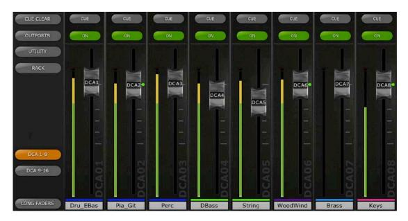
Press the [DCA 1-8] or [DCA 9-16] button again to exit the DCA fader bank and return to the previously selected bank. Alternatively, press any bank in the "Navigation/Meter Bridge" to directly access that fader bank.
