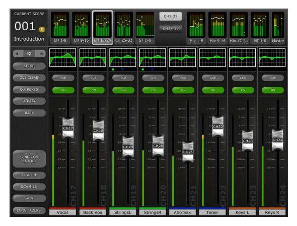
Across the top of the screen, level meters and faders are displayed in blocks of channels for mono Input Channels 1-32, Stereo Input Channels 1-8, Mix and Matrix busses, and the Master Stereo and Mono busses. This is the "Navigation/Meter Bridge".
