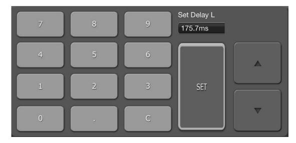
Tap the button to open the number keypad. Tap the Up/Down cursor buttons to adjust the parameter value one step at a time. The value will be sent to the console each time the cursor button is tapped.
