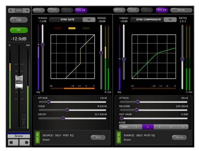
The left side of this screen (Channel Strip) is identical to the EQ Editing screen with channel fader, On button, Cue button, input and output meters, channel name, color and navigation buttons.
