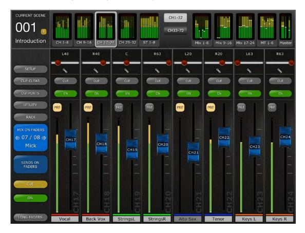
The large [MIX ON FADERS] button displays the currently selected Mix or Matrix Bus number and its name. The color of this button matches those used in the CL console.
