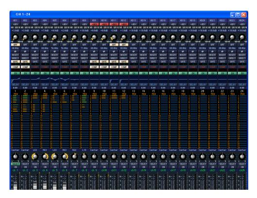
This window displays the mix parameters of input channels 1–24 or 25–48. The window shows either the channel 1–24 layer or the channel 25–48 layer. To open the other layer's window, choose the [Windows] menu command [INPUT CH] and choose "CH1-24" or "CH25-48."
