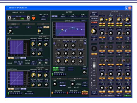
NOTE Unless otherwise specified, the parameters explained below are common to input channels 1–48, ST IN channels 1–4, and FX RTN channels 1–4.
