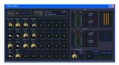
Here you can select the effect type for internal effects 1–8, edit the parameters, and specify the input/output patching.
