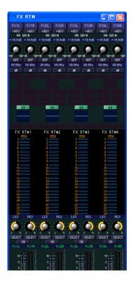
In this window you can view and edit the mix parameters of FX RTN channels 1–4. You can use the [View] menu to choose the parameters that will be displayed in the window.
