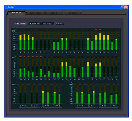
Here you can view the signal levels within the PM5D, or the amount of gain reduction produced by the internal compressors and gates. This lets you check signal presence, overload status, and compressor/gate operation from your computer. This window is divided into INPUT METER, OUTPUT METER, INPUT GR, and OUTPUT GR pages. To switch pages, click the tabs shown in the upper part of the window.
