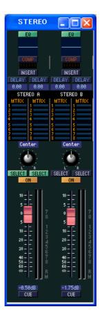
In this window you can view and edit the parameters of the STEREO A/B channels. You can use the [View] menu to choose the parameters that will be displayed in the window.
