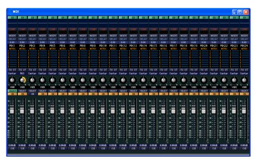
In this window you can view and edit the parameters of MIX channels 1–24. You can use the [View] menu to choose the parameters that will be displayed in the window.
