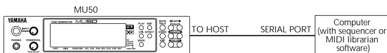
Bulk Dump data can be sent and received using the TO HOST connection.
