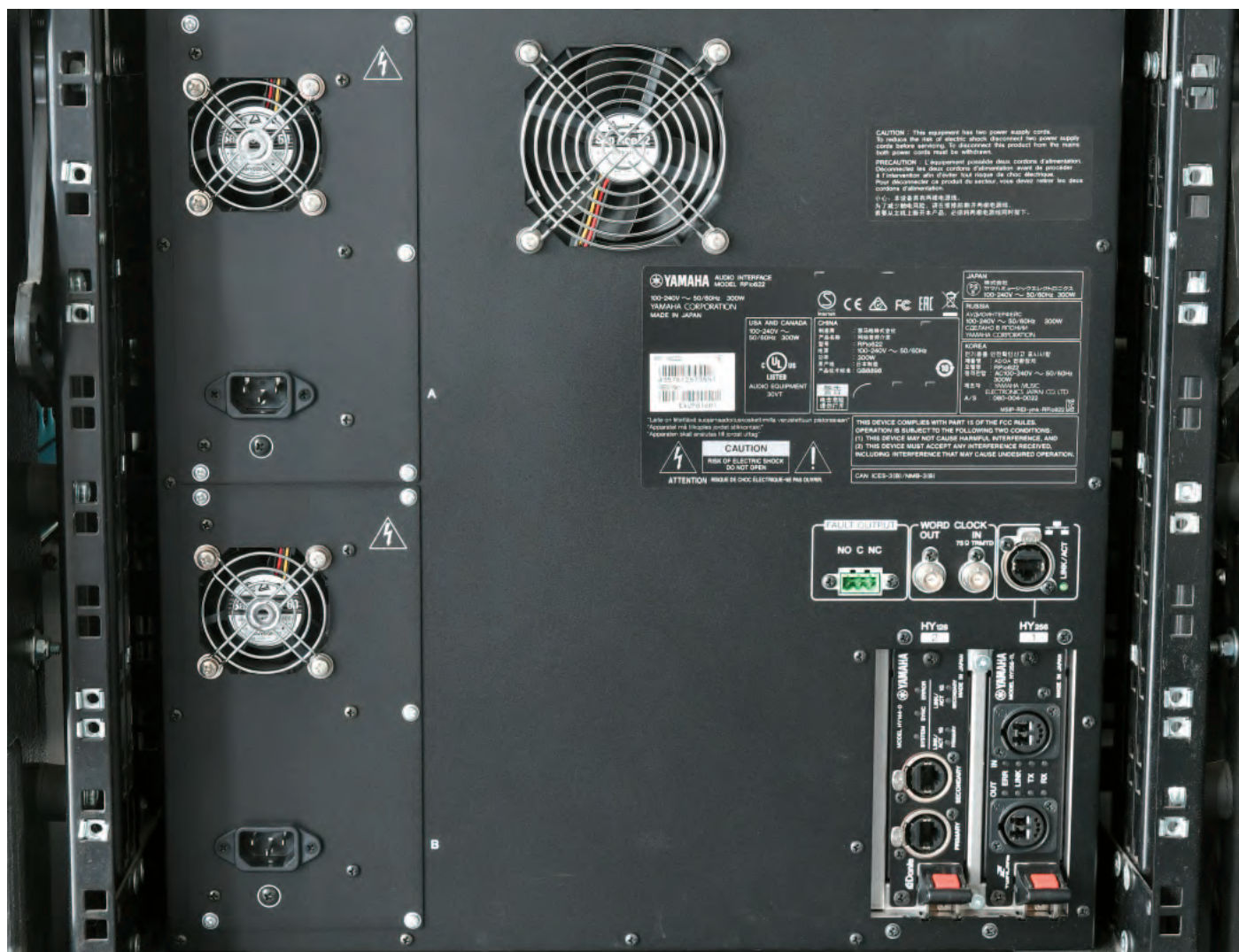
I/O rack RPio622 from the rear with two HY slots; also here one will find the obligatory two power supplies
