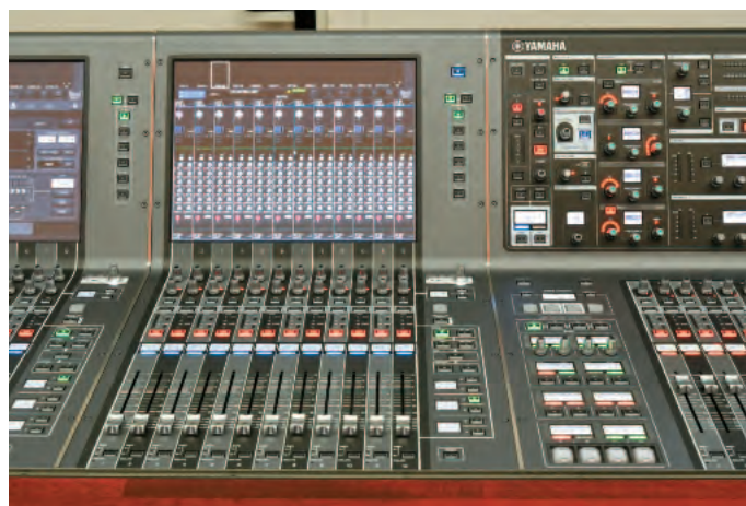
One of three 12-channel fader bays on the PM10 console's interface; the channel section can be seen in the top right of the picture
