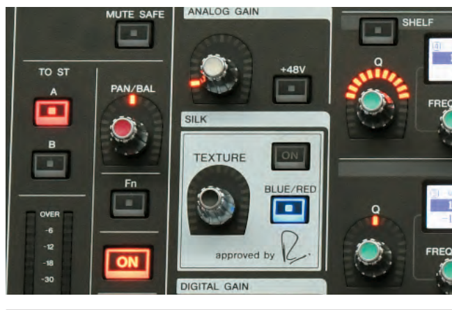
Silk setting with the selection “blue” for low-frequency and “red” for high-frequency as well as the texture setting for the intensity of the Silk processing
