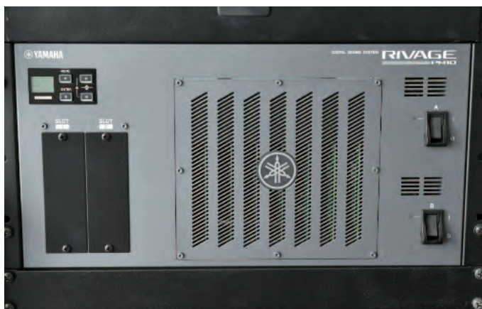
DSP engine from the front and rear. On the front side, there are two slots for cards in the familiar MY format. Up to four HY cards for TWINLANE or Dante cards can be used on the back. The HY cards can transmit up to 256 (TWINLANE) or 144 (Dante) channels. The DSP engine is of course equipped with two power supplies
